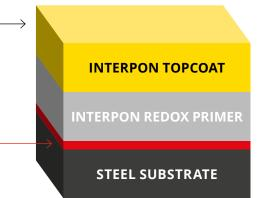
Interpon Redox powder systems enable you to perfectly meet specific protection requirements and application limitations for your project. After you have identified the corrosivity of the environment and the desired longevity of protection, selecting the right system takes three steps:
